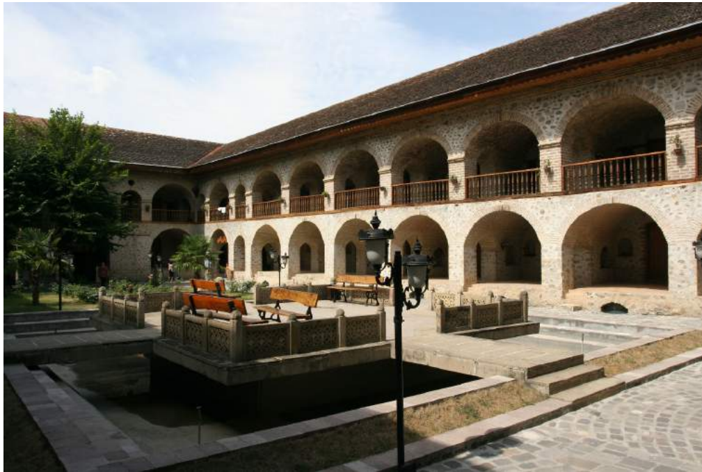
FIGURE 84: Arches are structural elements forming continuation of the walls, gates, doors, and windows and allowing the distribution of the load by dividing the structure diagonally.
