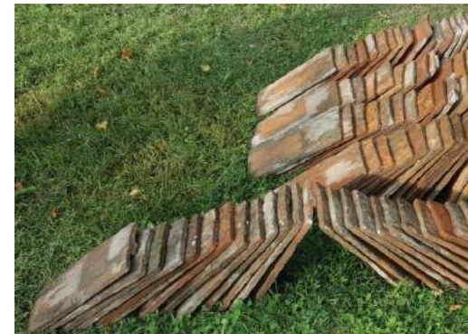
FIGURE 49: The roofs are covered with flat ceramic tiles in a parallel fashion. This type of roofing requires continuous maintenance.
