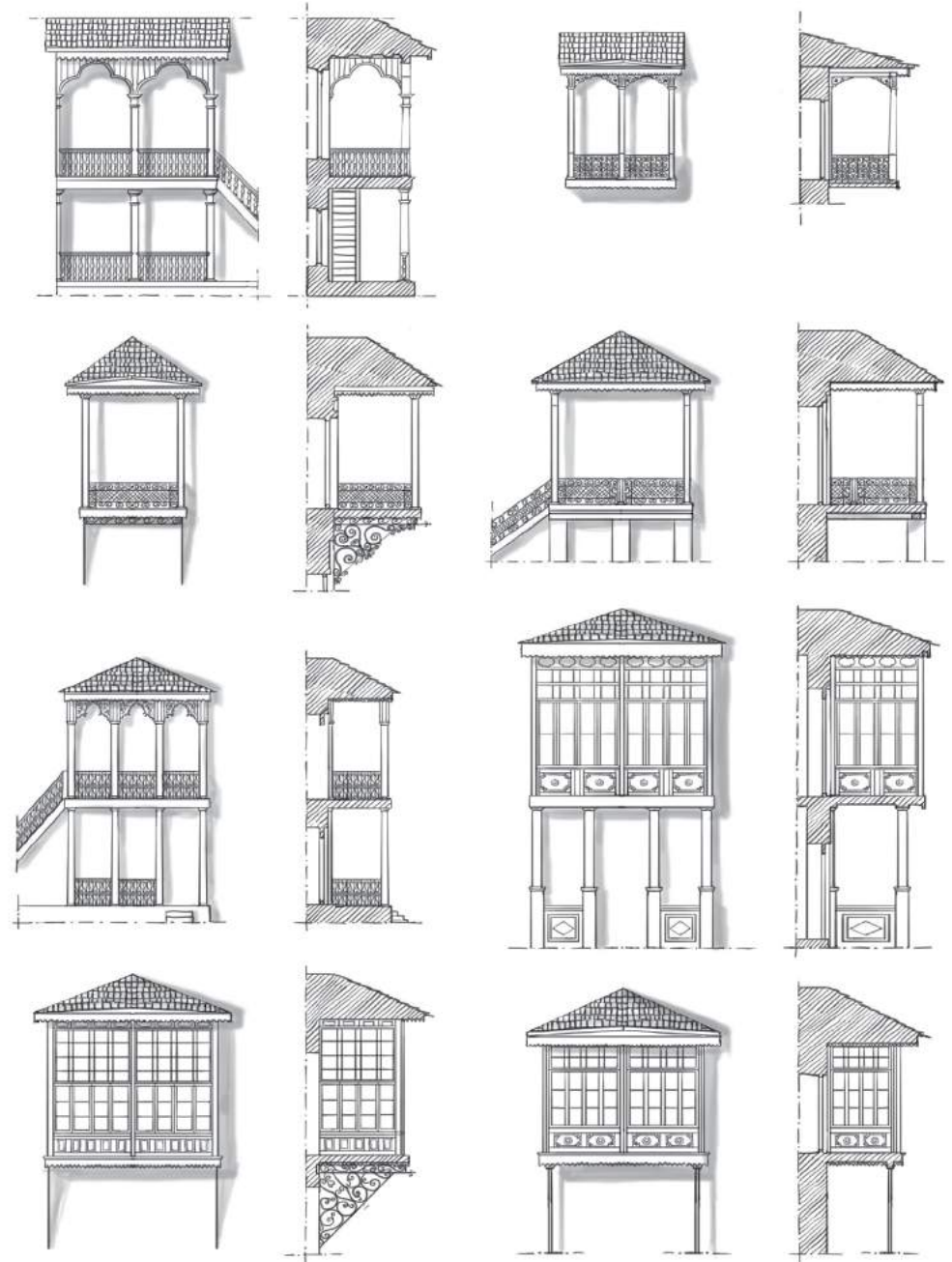
FIGURE 44: Traditional types of balconies. The open balconies are the oldest type.
