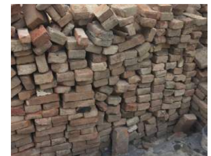
FIGURE 126: Fired bricks come in two colors, depending on the technology of firing and the amount of iron in them.
