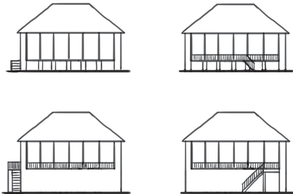
FIGURE 81: Traditional outdoor stairs in a straight run
